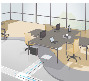
Screed floor system
