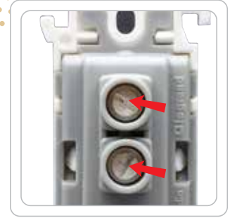
Finger-proof terminals for IP 20 protection against accidental contact
